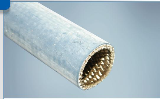
Ben-Har™ 1151-FRB Grade A is a rugged, flame-retardant, silicone rubber coated sleeving that provides excellent cut-through and abrasion protection for wiring systems in applications with temperatures ranging from -70°C to +200°C. Because the specially formulated silicone rubber is extrusion coated over the non-combustible fiberglass braid, it results in a reinforced sleeving that is superior to ordinary dip-coated sleeving and unreinforced rubber or plastic tubing.
