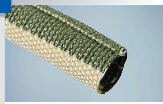
**ROUNDIT® 2000 NX HT** is a self-wrapping sleeve manufactured from PEEK monofilaments and Nomex® multifilaments. It includes a water repellent treatment in order to prevent the absorption of condensation build-up caused by the extreme changes aircraft are subjected to. Designed for mechanical protection and maintenance of wire and cable bundles, its 100% covering ratio provides excellent cut-through and abrasion resistance.
