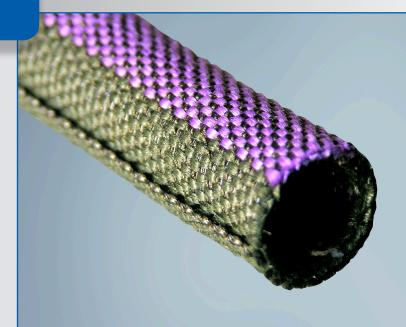
**ROUNDIT® 2000 NX VTR** is a woven combination of Nomex® and PPS (polyphenylene sulfide). The Nomex/PPS blend in a flat weave construction gives ROUNDIT 2000 NX VTR a rugged yet smooth texture and appearance for high temperature bundling and abrasion resistance. This product is rated to +200°C (+392°F) and is non-halogenated.
