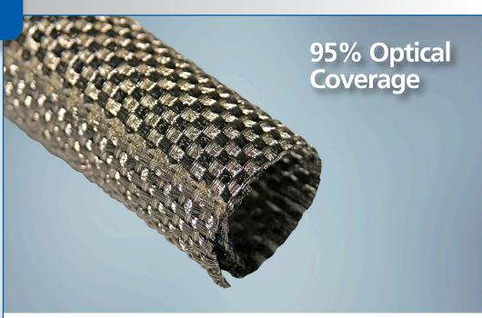
**ROUNDIT® EMI FMJ (Full Metal Jacket)** is a wrap-around sleeving designed for highperformance EMI shielding of wire and cable bundles. ROUNDIT EMI FMJ is manufactured from PPS monofilaments and nickel plated copper.
